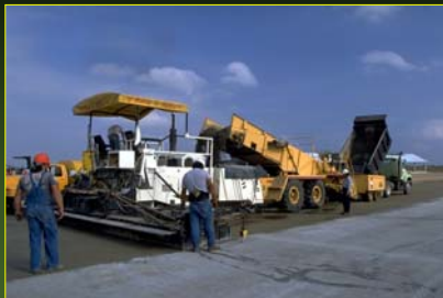
Transfer equipment keeps paver fully charged
